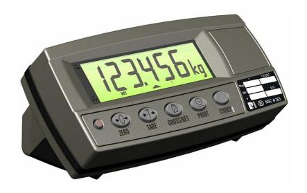
The R320 can power up to 4 x 350 Ohm load cells and is software selectable for either 4 wire or 6 wire operation (sense wire linking is not required).
