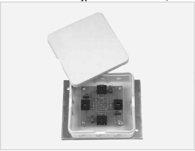
The plastic junction box is designed to connect 4 Type PB load cells in parallel. The box is mounted on an aluminium plate for proper mounting and shielding.
